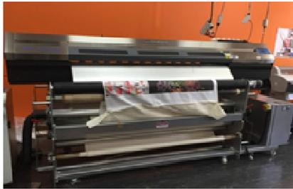
Figure 10: Digital Printing Machine – Roland Soljet III XJ-640
