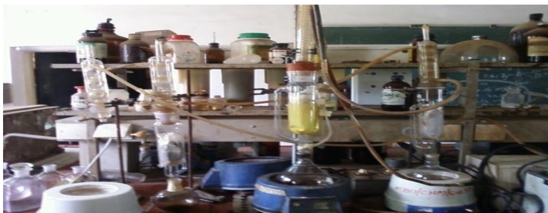
Plate 5: Rosigold mango kernel oil extraction with Soxhlet apparatus.
