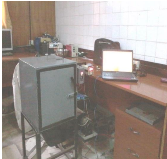
Figure 6: Dryer with Associated Instrumentation
