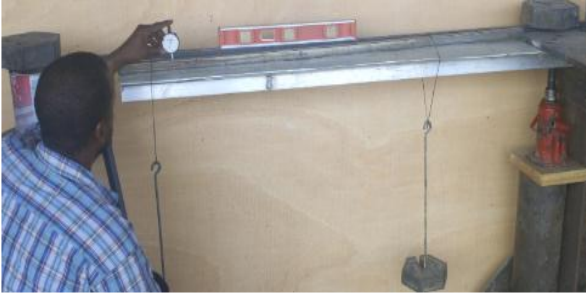
Figure 2. Experimental test of the blade structural material under load deflection condition
