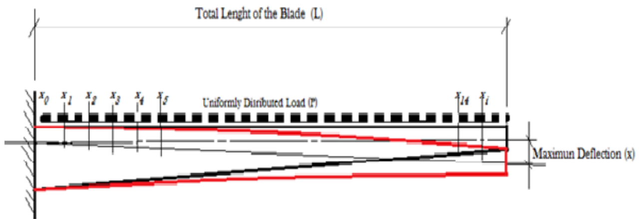
Figure 1. Schematic diagram of the blade as a cantilever with uniformly distributed load
