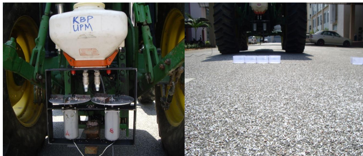
Figure 3: Arrangement of trays for granular fertilizer collection
