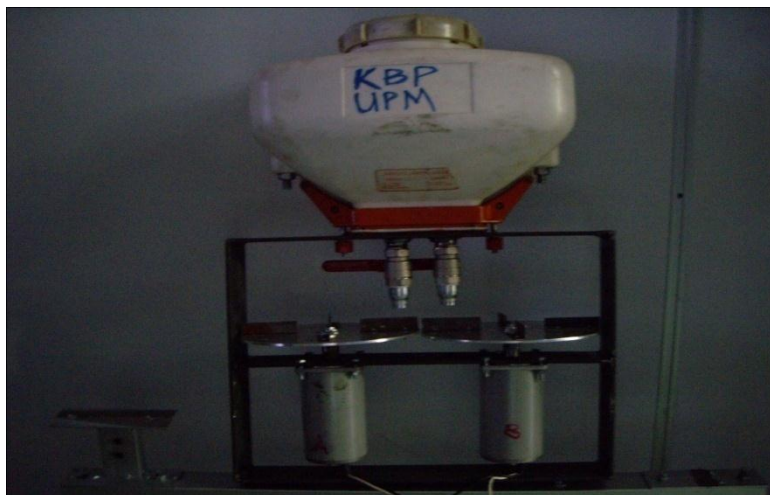
Figure 2: Photograph of the dual-purpose disc chemical applicator
