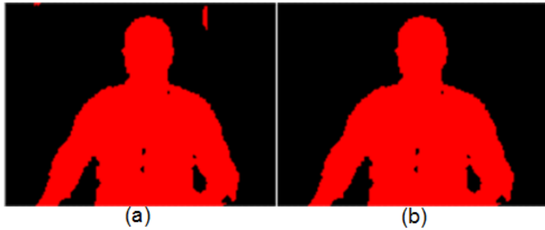
Figure 3: Binary image (a) containing little background objects and (b) objects removed
