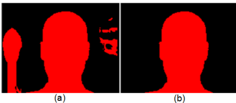
Figure 7: Binary image (a) containing multiple background objects and (b) objects removed
