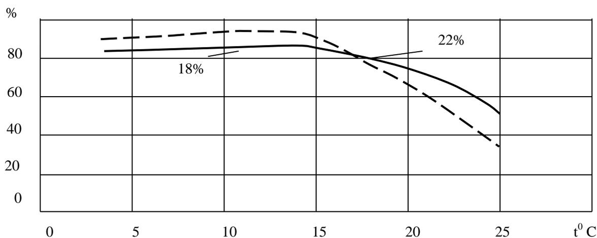
Figure 3. The relationship between the percentage of HS<sup>-</sup> in the sea water and the temperature P=10<sup>5</sup> Pa.
