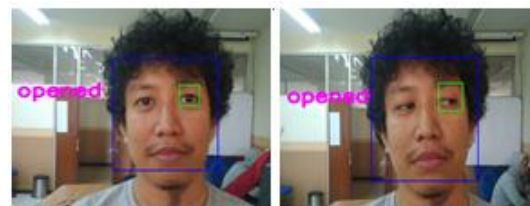
Figure. 14 Blink detection using our proposed method that not affected by pupil position
