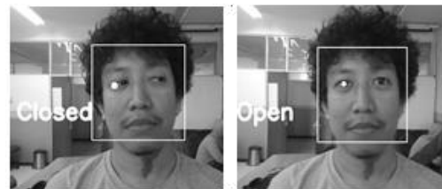
Figure. 13 Blink detection using Contour Circle method. wrong detection caused by pupils are not in the center (left)
