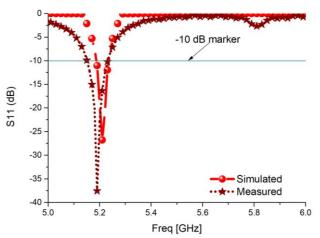
Figure. 7 Simulated and measured S11 parameter
