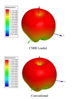
Figure. 9 Simulated gain 3D-polar plot of CSRRs loaded and conventional antenna
