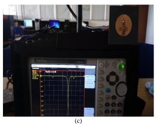
Figure. 6 Prototype and measurement setup: (a) top view of the prototype, (b) bottom view of the prototype, and (c) S11 measurement setup
