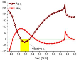
Figure. 5 Dielectric constant of CSRR loaded antenna structure
