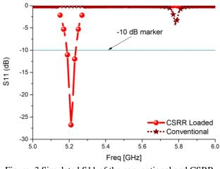
Figure. 3 Simulated S11 of the conventional and CSRR loaded antennas
