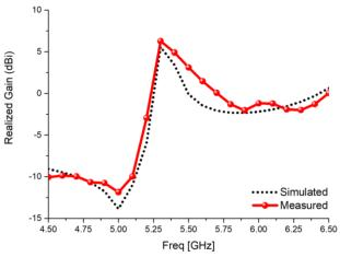
Figure. 8 Simulated and measured realized gain
