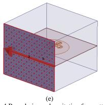
Figure. 4 Boundaries and excitation for scattering parameter inversion method: (a) antenna into the air box, (b) perfect E-field to a pair of horizontal faces, (c) perfect H-field to the pair of horizontal faces, (d) master-slave 1, and (e) master-slave 2
