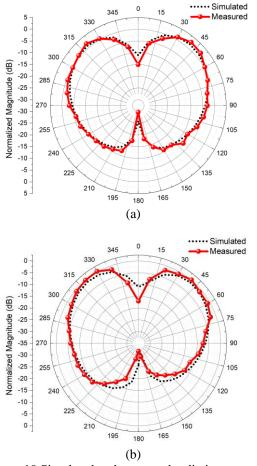
Figure. 10 Simulated and measured radiation pattern: (a) E-plane and (b) H-plane
