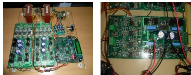
Figure.10 Hardware model of the proposed inverter: (a) Structure of FPGA controller with the power circuit and (b) Internal power circuit and driver Circuit for H-bridge module
