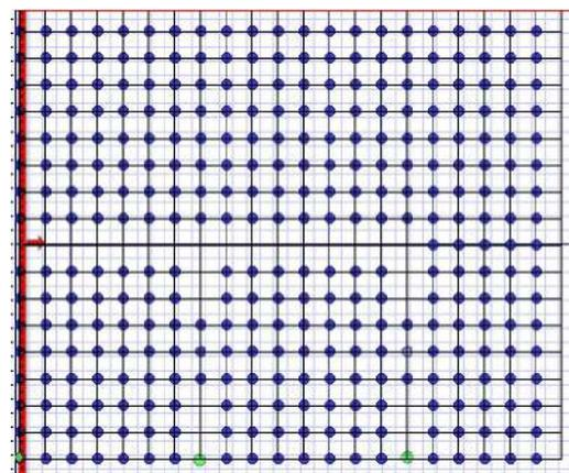
Fig.1 2D Photonic crystal based biosensor layout
