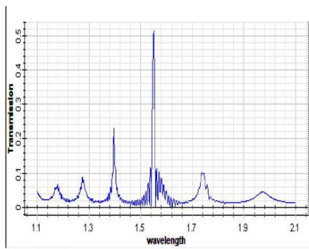
Fig. 5 Transmitted spectrum with refractive index (1.49)
