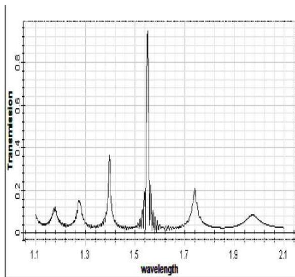
Fig 4: Transmission spectrum with refractive index (1.42)
