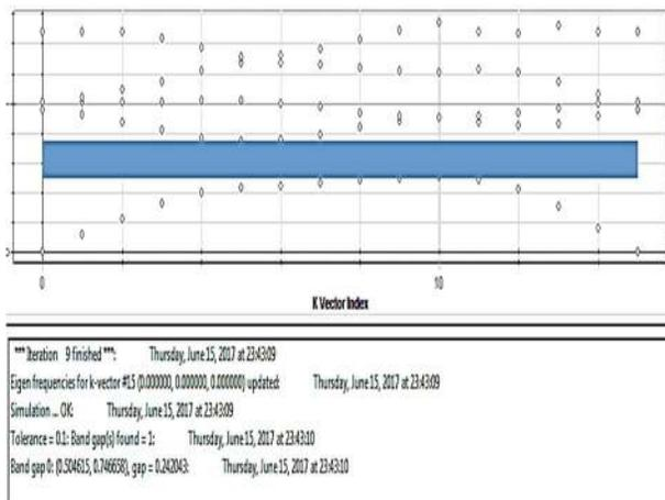
Fig.2 TE band diagram square lattice
