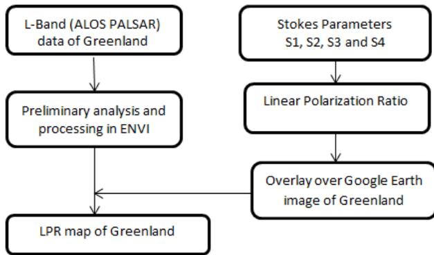
Fig. 2 Methodology to study LPR values of L-band for Greenland ice sheets
