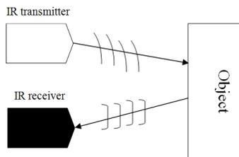
Fig 4: working of an IR sensor
