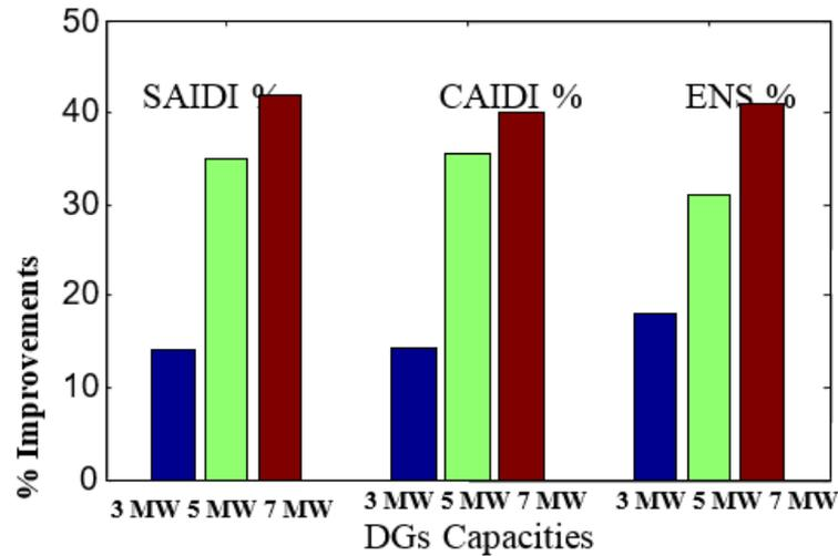
**Fig. 7** – % Improvements of reliability indices with DGs (3MW & 1\*3 MW)
