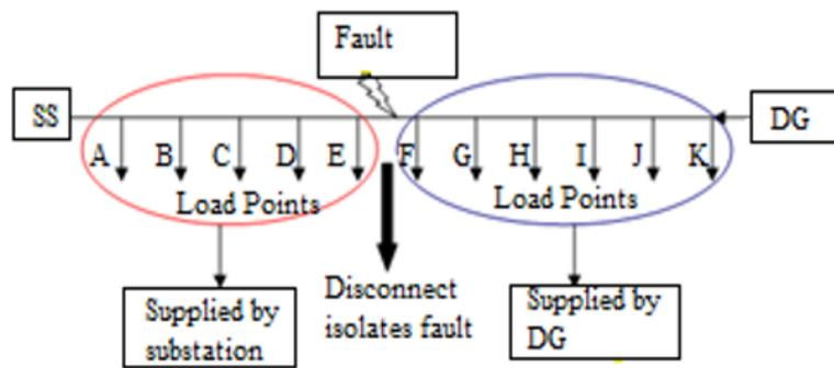
**Fig. 4** – Distribution system supplied with DG
