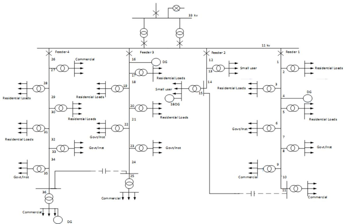
Fig. 5 – Distribution System for RBTS Bus 2
