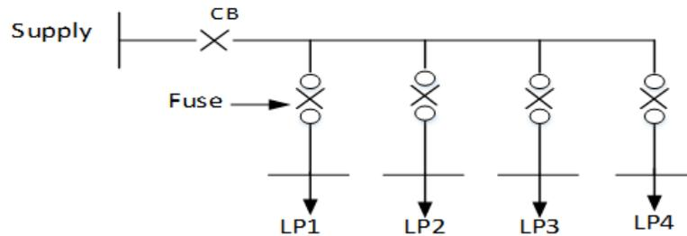
**Fig. 2** – A simple radial system with no disconnects on the main line
