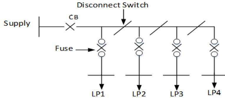
**Fig. 3** – A Simple radial system with disconnects on the main line
