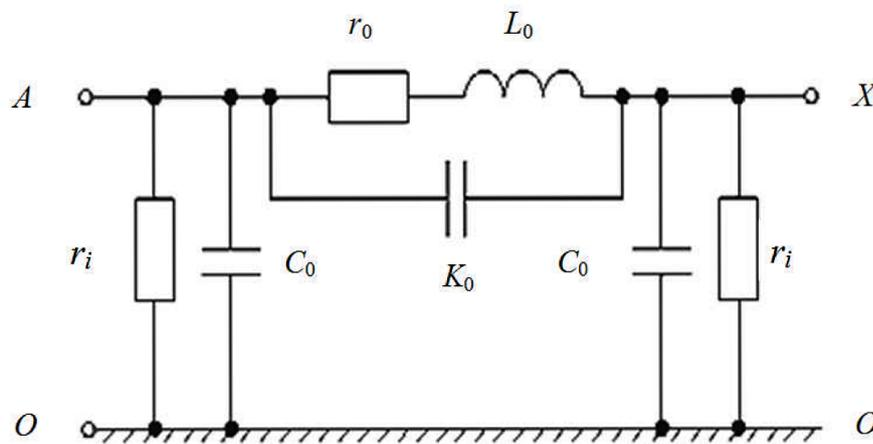
**Fig. 2** – Equivalent circuit of coil.
