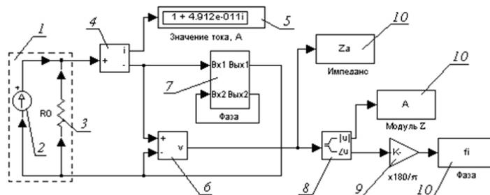
Fig. 12 – Simulation scheme related to the definition of longitudinal.
