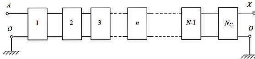
**Fig. 1** – Ladder circuit with  $N_c$  coils of motor phase.
