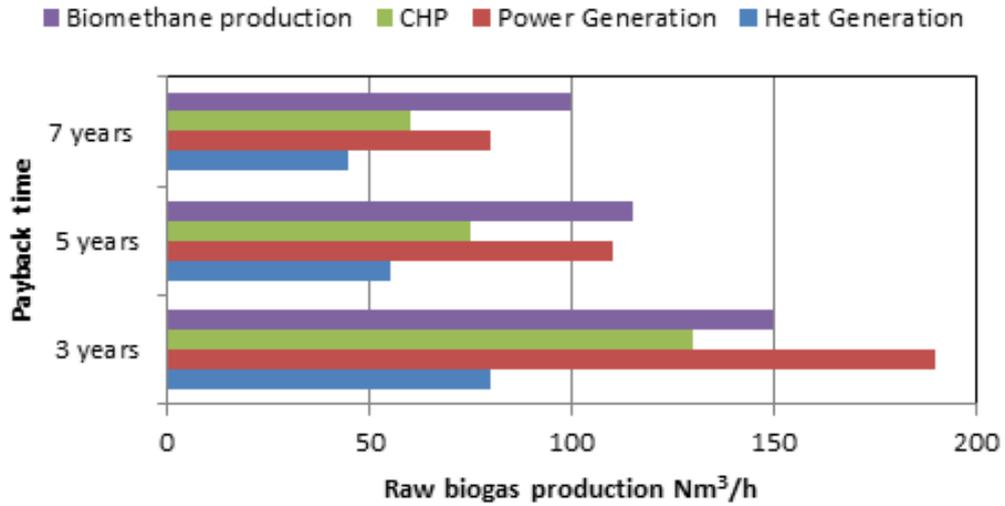
Fig. 4 – The payback time for the proposed valorization ways.
