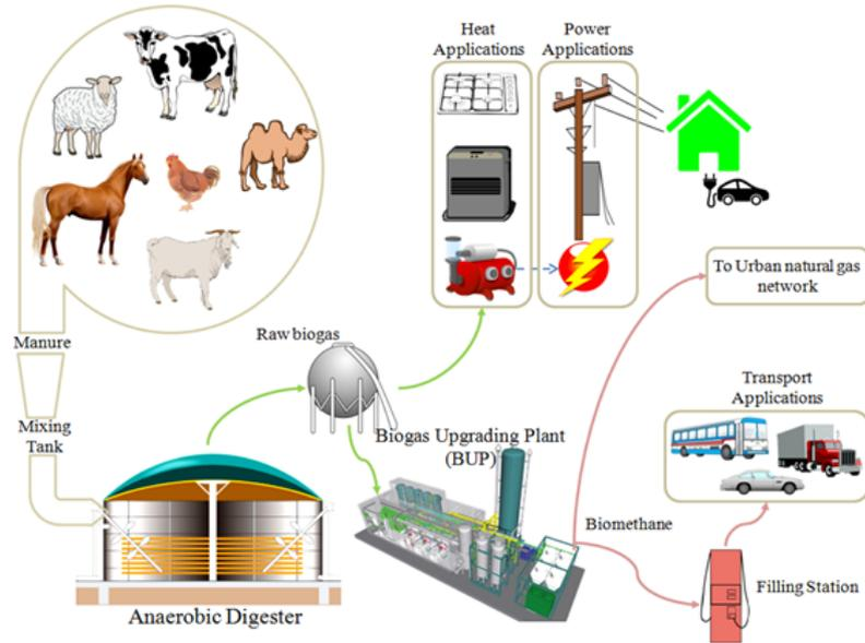
Fig. 1 – Summary of biogas production and Applications.
