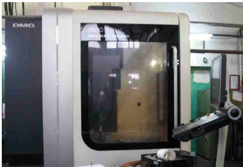
Figure 3. Vertical milling machine in three axes DMC 635v
