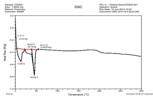
**Fig. 8: DSC thermogram of oxidized ghee**
