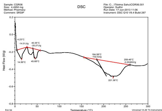
**Fig. 10: DSC thermogram of rosuvastatin calcium:Oxidized ghee complex (1:1)**
