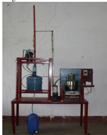
Figure 1. The prototype waste plastic oil converter
