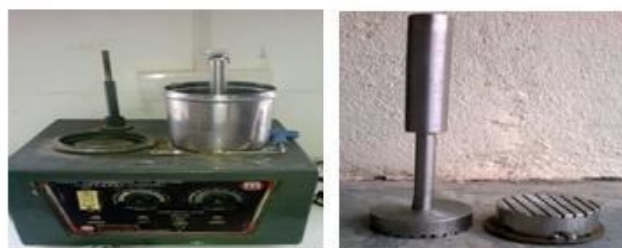
Figure 2: Lab fabricated Medicated Chewing Gum apparatus with Die and punch.
