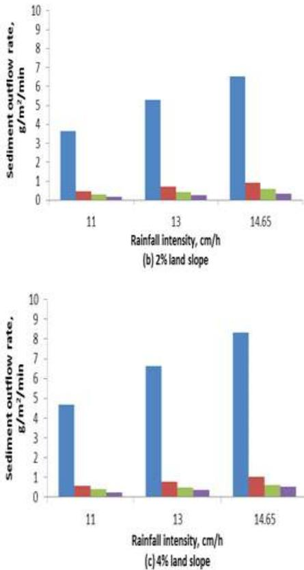
Fig. 7 : Comparison of sediment outflow rate for different paddy straw mulch at different rainfall intensities and land slopes
