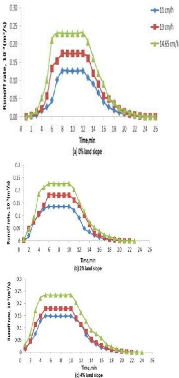
Fig. 5 : Observed runoff hydrograph at different land slopes and rainfall intensities for 10 ton/ha paddy straw mulch
