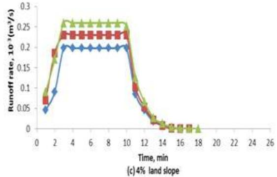
Fig. 2 : Observed runoff hydrograph at different land slopes and rainfall intensities for no mulch
