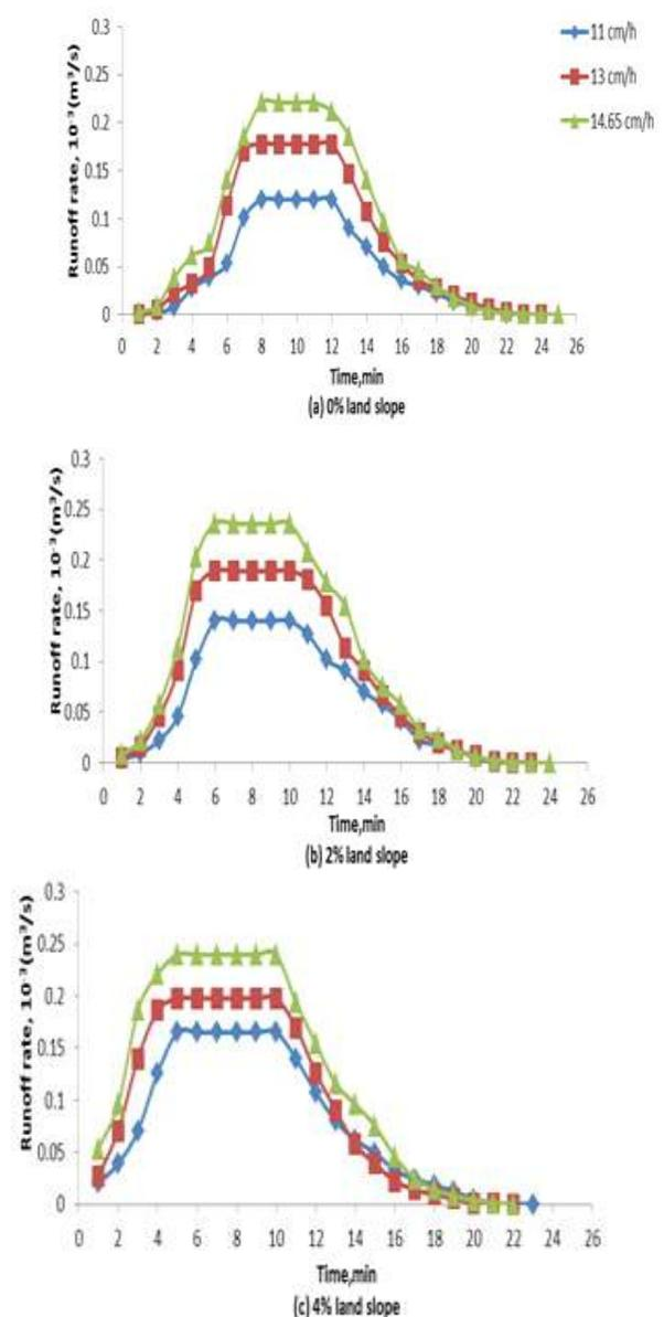
Fig. 4 : Observed runoff hydrograph at different land slopes and rainfall intensities for 8 ton/ha paddy straw mulch
