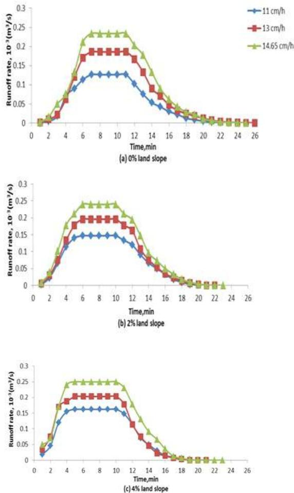
Fig.3 : Observed runoff hydrograph at different land slopes and rainfall intensities for 6 ton/ha paddy straw mulch
