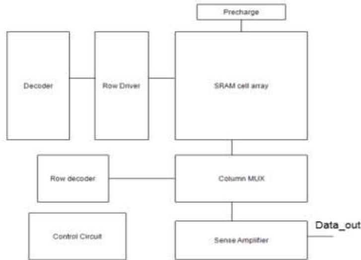
Fig 1: Block diagram of SRAM memory array
