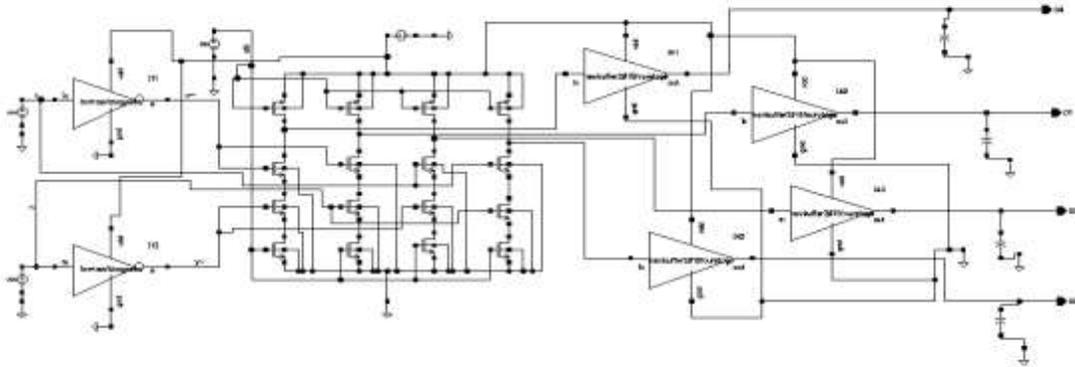
Fig 4: Integration of dynamic NAND 2:4 decoder with four stage CMOS taper with bypass buffer
