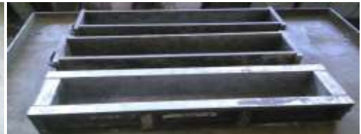
Figure 2(c) Beam Moulds
