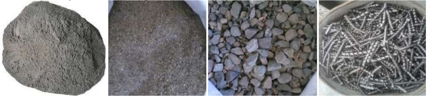
Fig 1: Cement, Course Sand, Course Aggregate and Lathe machine scrap from left to right respectively
