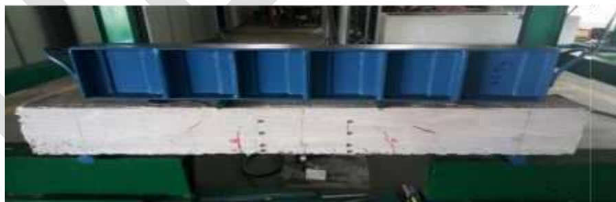
Fig.2 Experimental setup of beam specimen
