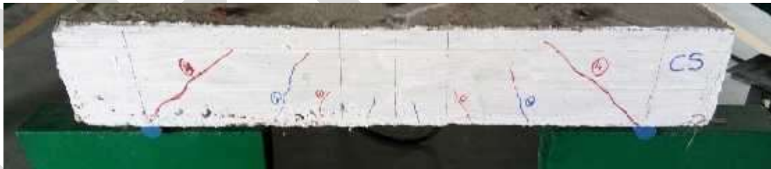
Fig 9. Crack pattern for control specimen
