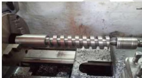
Fig 2: Helical groove cutting process.
