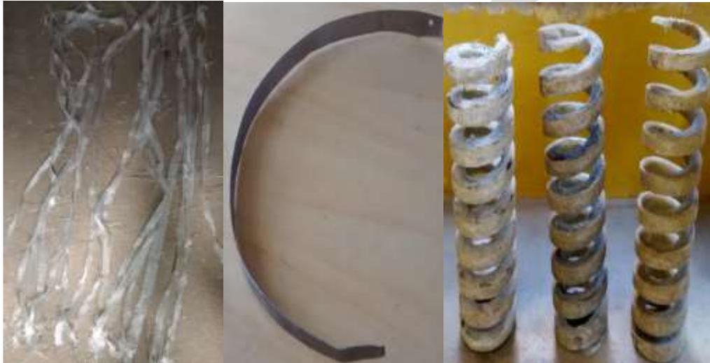
Fig 4: Fiber and steel strip with 90° orientations
