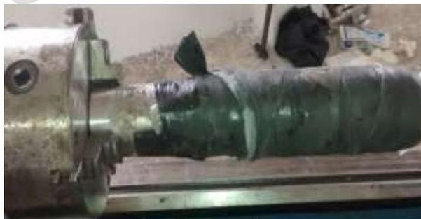
Fig 3: Tube strip wound on mandrel
