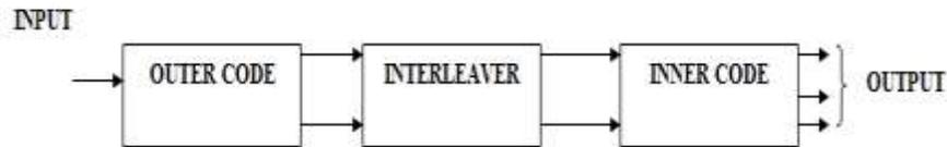
Fig 4: Serial Concatenated Convolutional Codes (sccc) [2]
