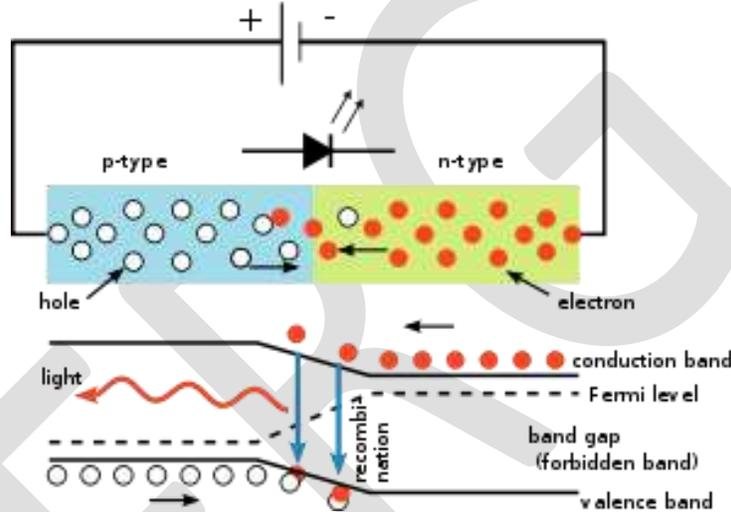
Fig 1. Circuit and Band Diagram of LED.
