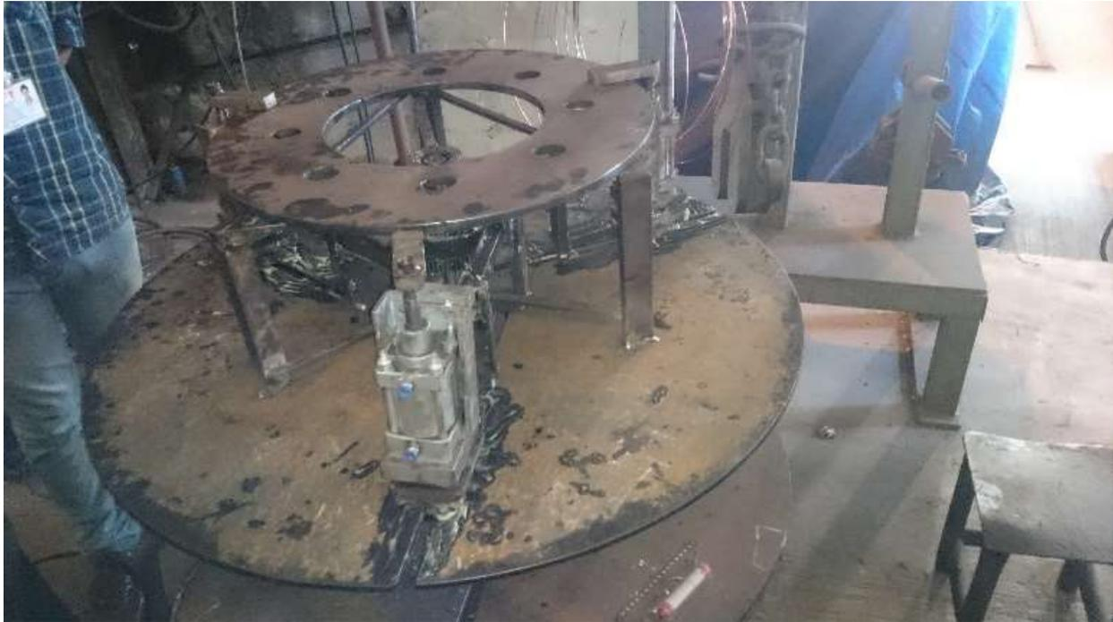
Figure 7. Self-Centering Mechanism with plate
