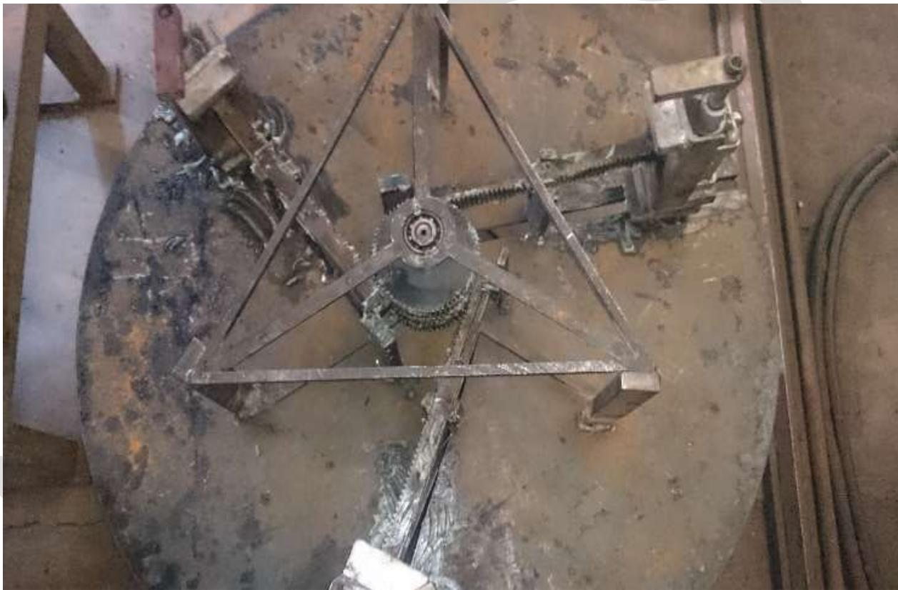
Figure 6. Self-Centering Mechanism without plate
