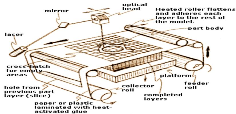
Material is usually a paper sheet laminated with adhesive on one side, but plastic and metal laminates are appearing.
