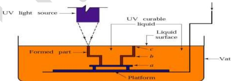
In new SL systems, a blade spreads resin on the part as the blade traverses the vat. This ensures smoother surface and reduced recoating time.
