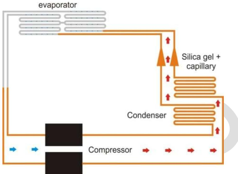
**Fig. 1 Schematic diagram of Refrigeration Cycle (VCRS)**
