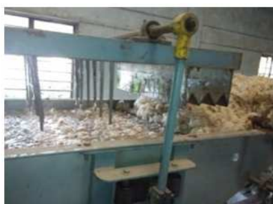
Figure 5: Two Bowl Scouring of UAS Sheep Breed Wool Fibres
