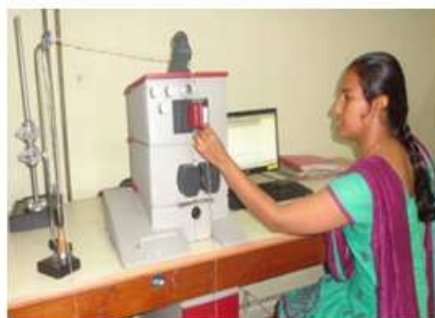
Figure 10: Yarn Evenness Testing of the Pure UAS Sheep Breed Wool and Blended Yarns
