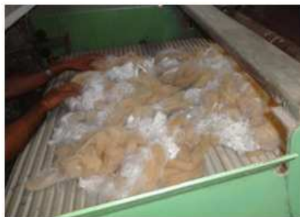
Figure 7: Feeding UAS Sheep Breed Wool Blended Fibres in to the Woolen Card
