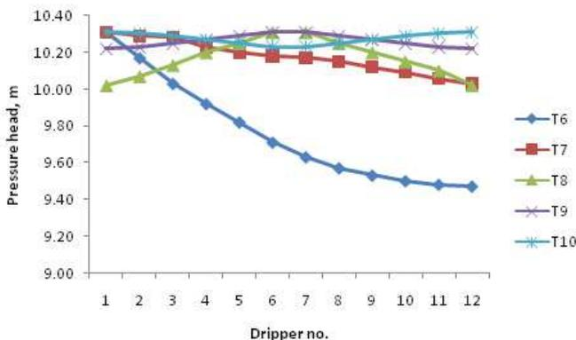
Figure 2: Ariation of Pressure along the Lateral in Different Lateral Connections (Sub-Main Size 50 mm)
