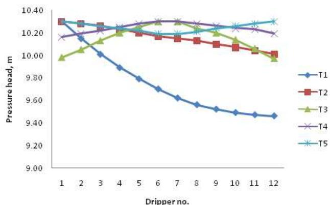
Figure 1: Ariation of Pressure along the Lateral in Different Lateral Connections (Sub-Main Size 40 mm)
