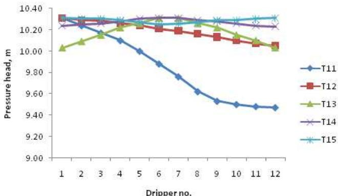
Figure 3: Ariation of Pressure along the Lateral in Different Lateral Connections (Sub-Main Size 63 mm)
