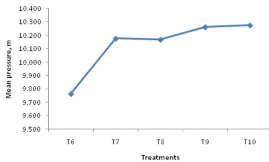
Figure 5: Ariation of Mean Pressure as Affected by Different Treatments (Sub-Main Size 50 mm)
