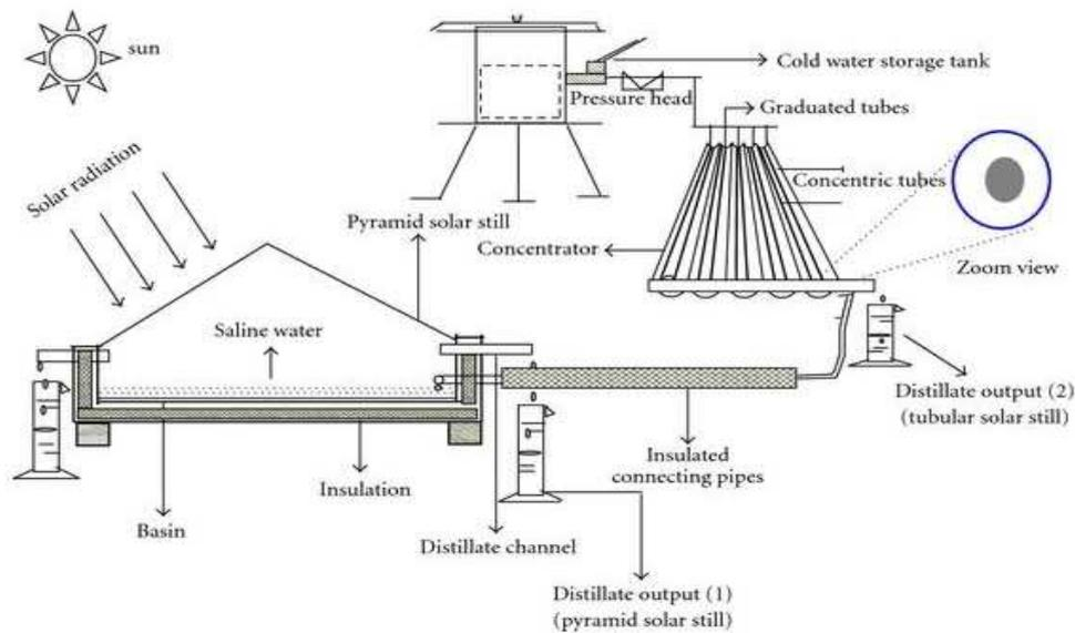
**Figure 5: Cross Sectional View of Coupled Tubular and Pyramid Solar Still.**
