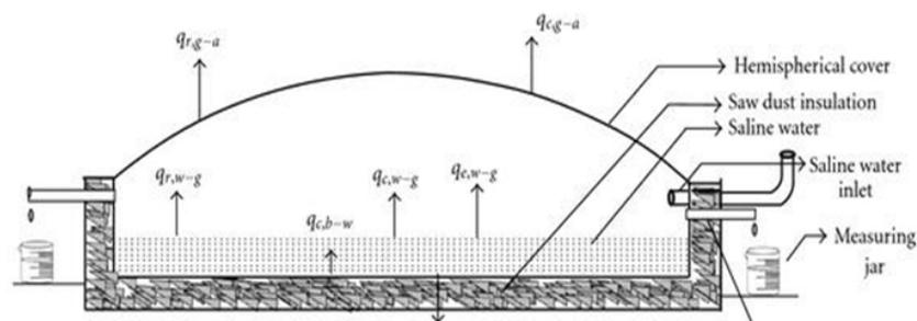
**Figure 4: Schematic View of Solar Still of Hemispherical Form**
