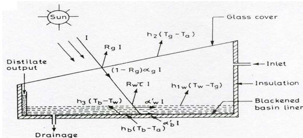
Figure 1: Diagram of a Conventional Single Slope Solar Still
