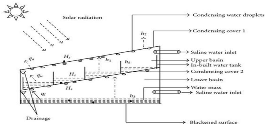
**Figure 3: The Cross-Sectional View of Solar Still Has Double Basin Glass**
