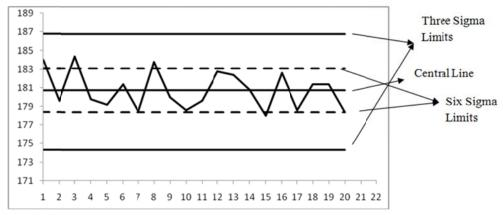
Figure 2. Six Sigma-based and traditional X-bar control charts
