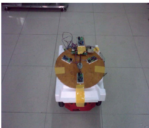
Figure.11 The mobile robot with the proposed acoustic localization system.
