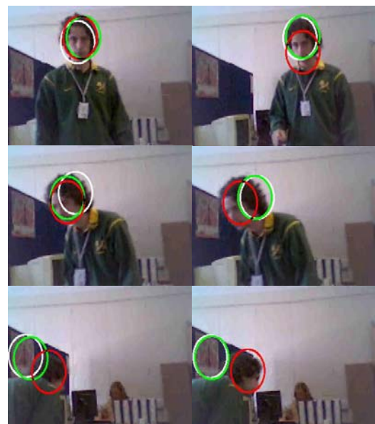
Figure.6 Rapid rotation sequence: The frames 62,68,87,88,101 and 102 are shown (left-right, top-down). The white, green and red circles show the tracking result of conventional mean shift algorithm, MSI I , and MSI II respectively.
