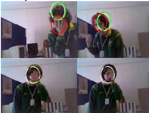
Figure.8 Occlusion sequence: The frames 38,103,121 and 123 are shown (left-right, top-down). The white, green and red circles show the tracking result of conventional mean shift algorithm, MSI I , and MSI II respectively.
