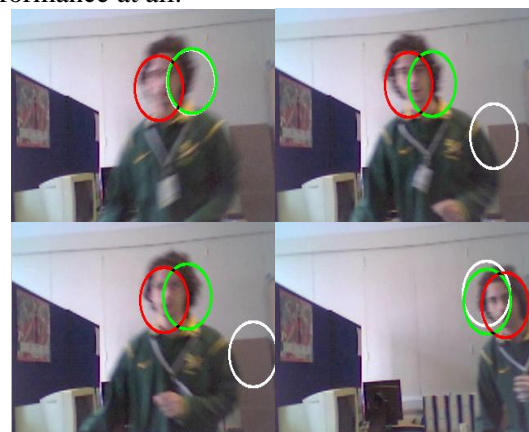
Figure.3 Rapid movement sequence: The frames 58, 63, 67 and 87 are shown (left-right, top-down). The white, green and red circles show the tracking result of conventional mean shift algorithm, MSI I, and MSI II respectively.
