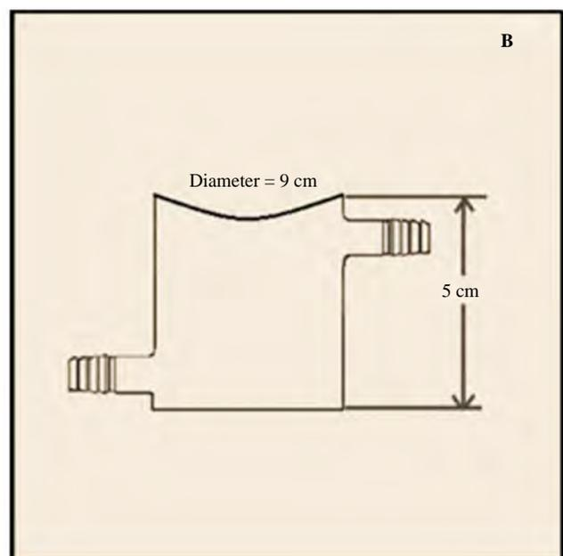
Figure 2. Glass feeder design B.
