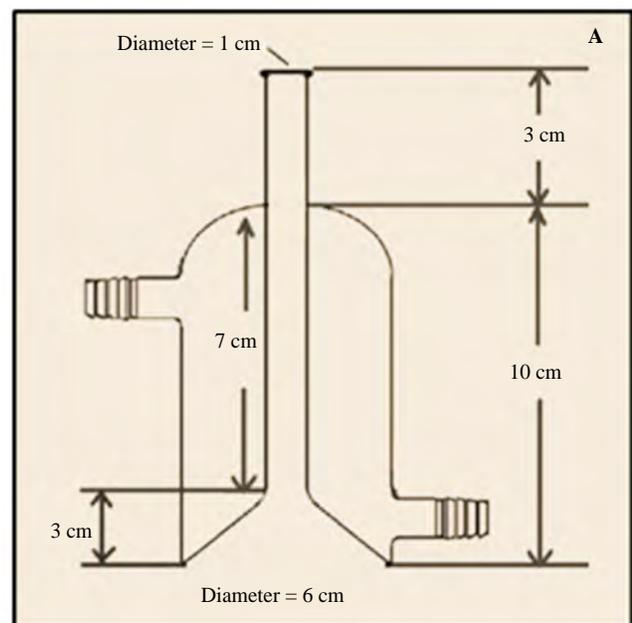
Figure 1. Glass feeder design A.
