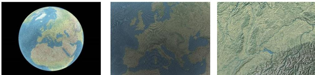
Figure 1. From left to right: Zoom into a 3D point cloud of earth data with 1 billion points (file size is 42.2 GB). Our proposed technique provides a smooth exploration on a standard computer system
