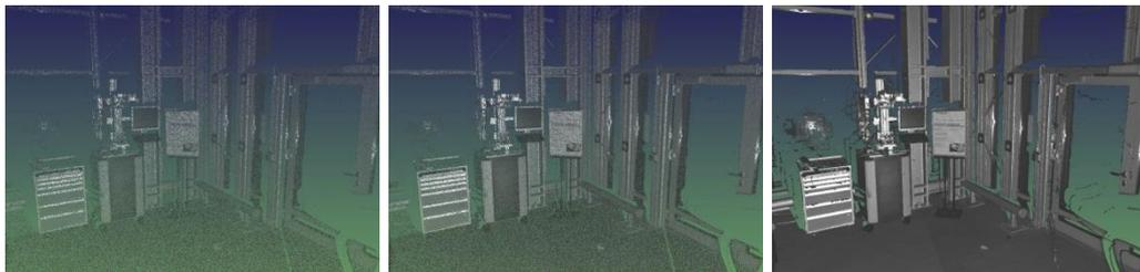
Figure 6. Detail accumulation for 650M points: Overview data is always rendered (left). If the camera is not moved, details are accumulated (middle and right image) whereat the transition is blended smoothly at constant time intervals
