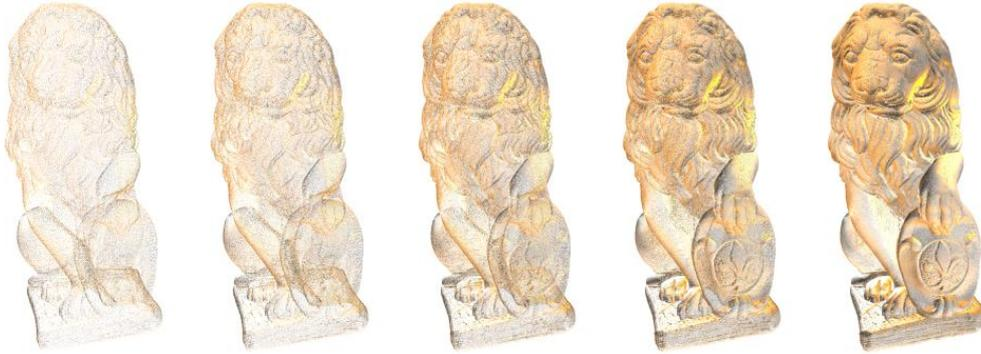
Figure 2. Overview point cloud with various point counts, starting with 125000 points (left) and doubled until 2 million points (right). The kd-tree ensures a well suited representation of the scanned volume at each point count limit
