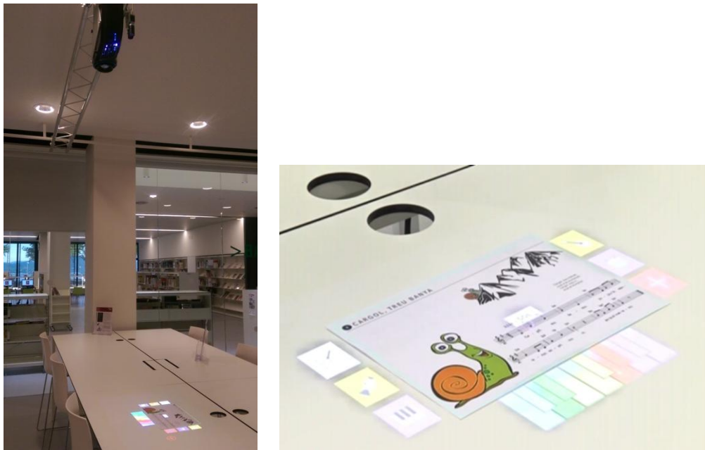
Figure 11. Left: Fixed setup in a public library. The fixed setup has the projector/camera pair fixed in a structure that is attached to the ceiling. This way, the users have free space around them to experiment and freely perform gestures to interact with the application. Right: The music toy application
