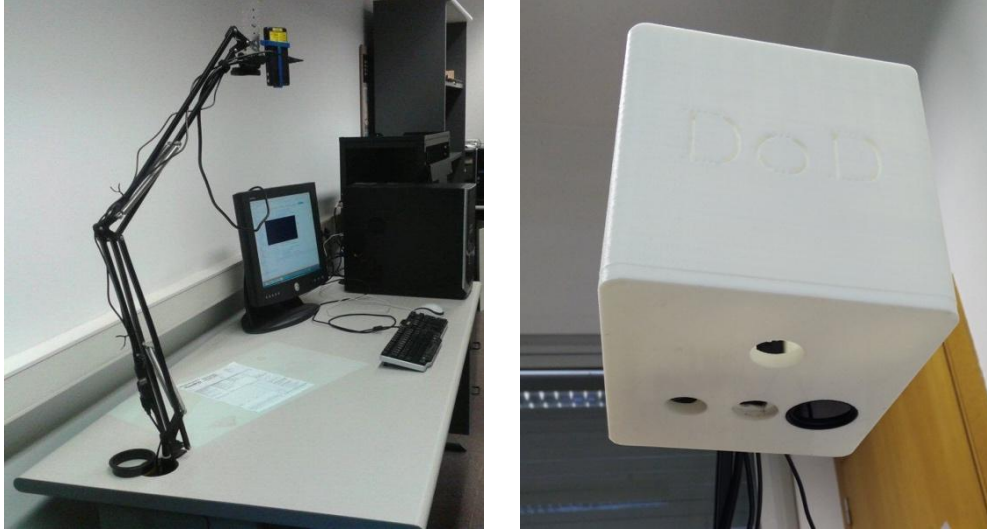
Figure 10. The initial setup of the nomadic system and the 3D printed shell to enclose the cameras and projector
