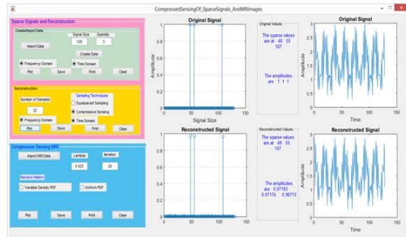
**Figure 9** The Reconstruction with Compressive Sensing Algorithm
