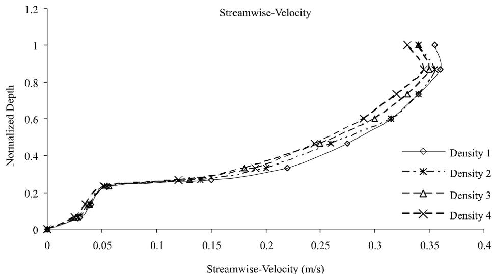
FIG. 3. STREAM-WISE VELOCITY PROFILES OVER THE DEPTH OF THE FLOODPLAIN
