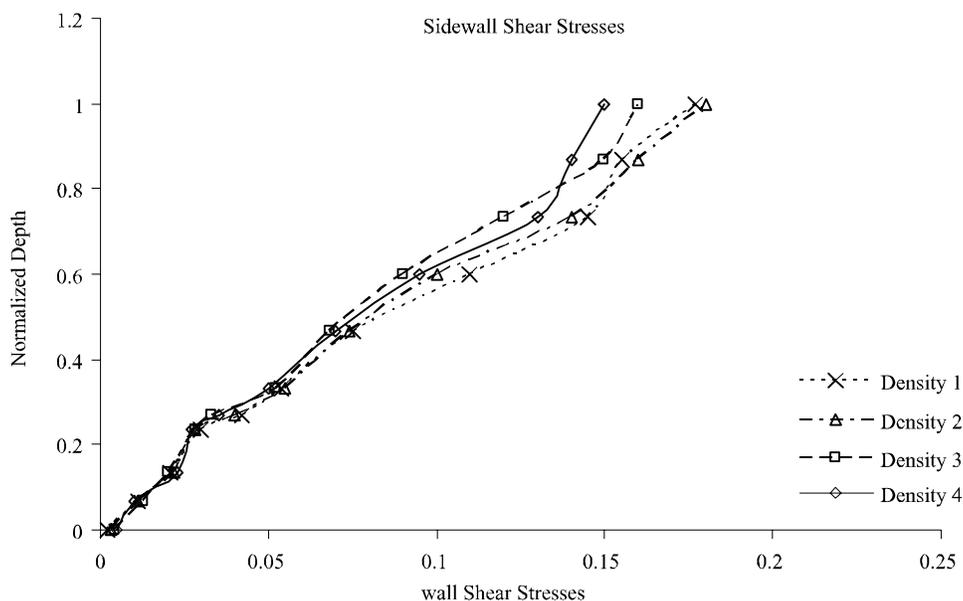
FIG. 6. SIDE WALL SHEAR STRESSES OF FLOODPLAIN
