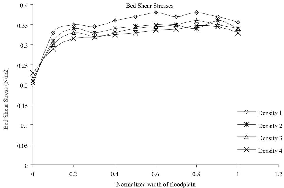
FIG. 5. BED WALL SHEAR STRESSES OVER THE WIDTH OF THE FLOODPLAIN
