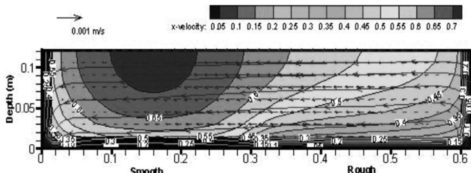
FIG. 7(c). PRIMARY VELOCITY CONTOURS AND SECONDARY VELOCITY VECTORS
