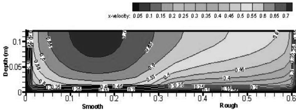
FIG. 7(a). PRIMARY VELOCITY CONTOURS
