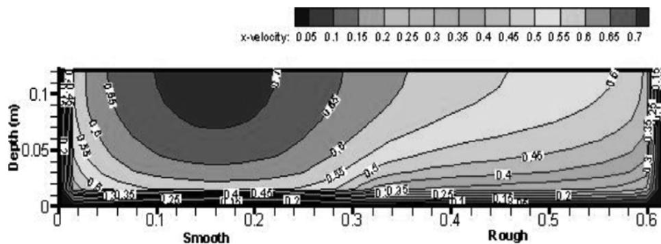
FIG. 7(a). PRIMARY VELOCITY CONTOURS
