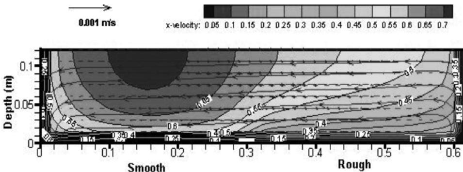
FIG. 6(c). PRIMARY VELOCITY CONTOURS AND SECONDARY VELOCITY VECTORS
