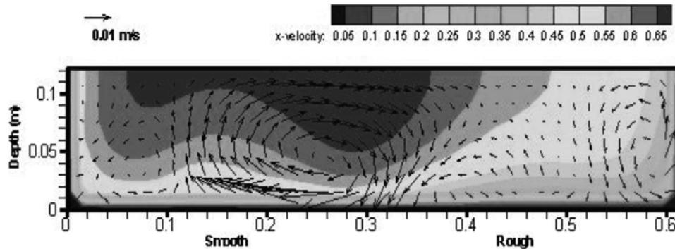
FIG. 5. PRIMARY VELOCITY CONTOURS AND SECONDARY VELOCITY VECTORS
