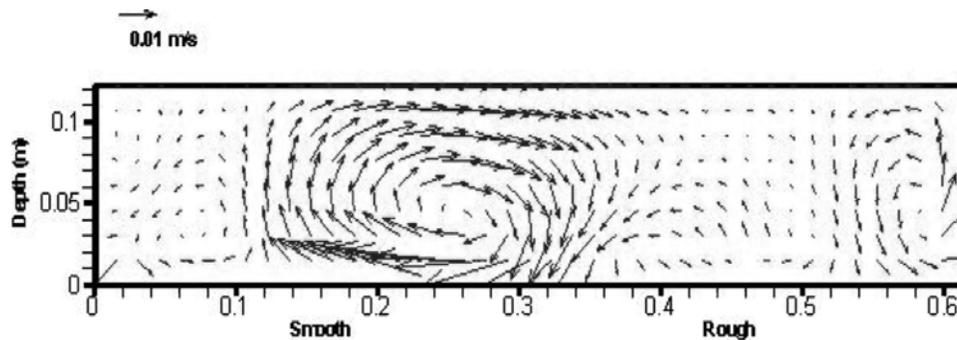
FIG. 4(b). SIMULATED SECONDARY VELOCITY VECTORS
