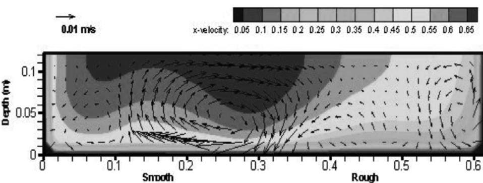
FIG. 5. PRIMARY VELOCITY CONTOURS AND SECONDARY VELOCITY VECTORS
