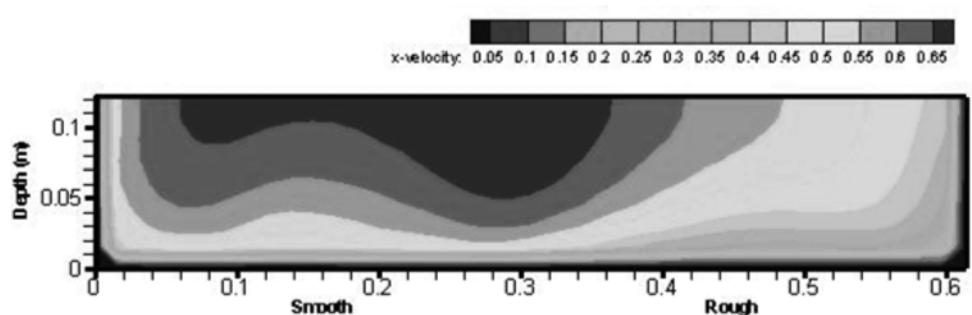
FIG. 3(b). SIMULATED PRIMARY VELOCITIES
