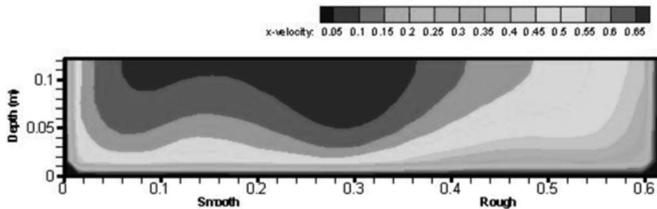
FIG. 3(b). SIMULATED PRIMARY VELOCITIES
