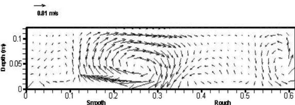
FIG. 4(b). SIMULATED SECONDARY VELOCITY VECTORS
