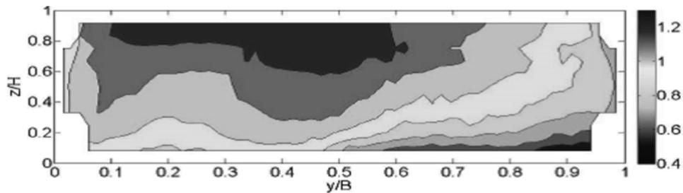
FIG. 3(a). EXPERIMENTAL PRIMARY VELOCITIES
