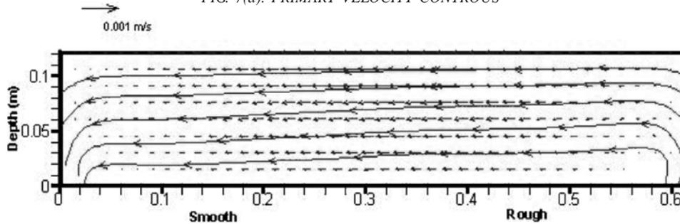
FIG. 7(b). SECONDARY VELOCITY VECTORS
