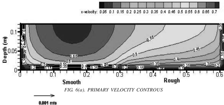
FIG. 6(a). PRIMARY VELOCITY CONTOURS
