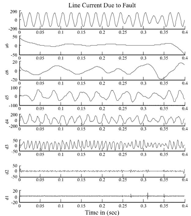
FIG. 4. LINE CURRENT FAULT TRANSIENT SIGNAL WITH  $D_1$ - $D_6$  DETAIL AND APPROXIMATION  $A_6$  COEFFICIENTS
