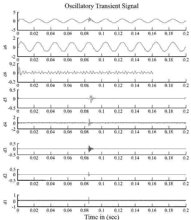
FIG. 1. OSCILLATORY TRANSIENT SIGNAL WITH  $D_1$ - $D_6$  DETAIL AND APPROXIMATION  $A_6$  COEFFICIENTS
