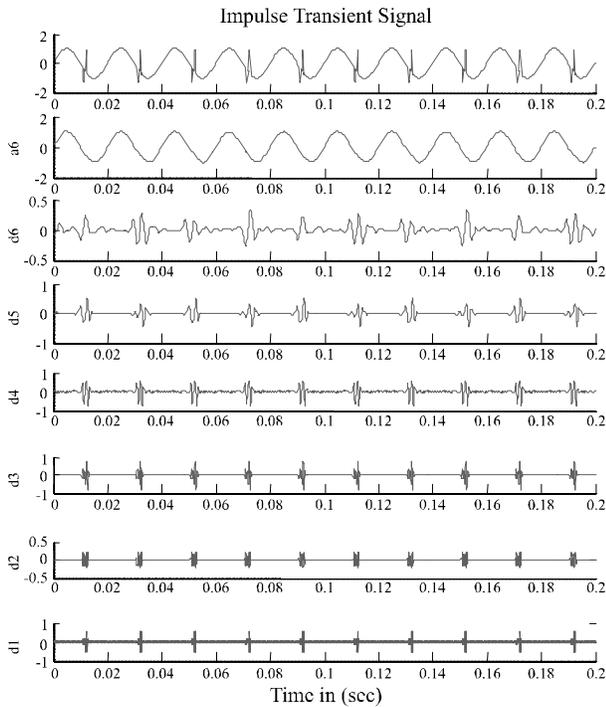
FIG. 2. IMPULSE TRANSIENT SIGNAL WITH  $D_1$ - $D_6$  DETAIL AND APPROXIMATION  $A_6$  COEFFICIENTS
