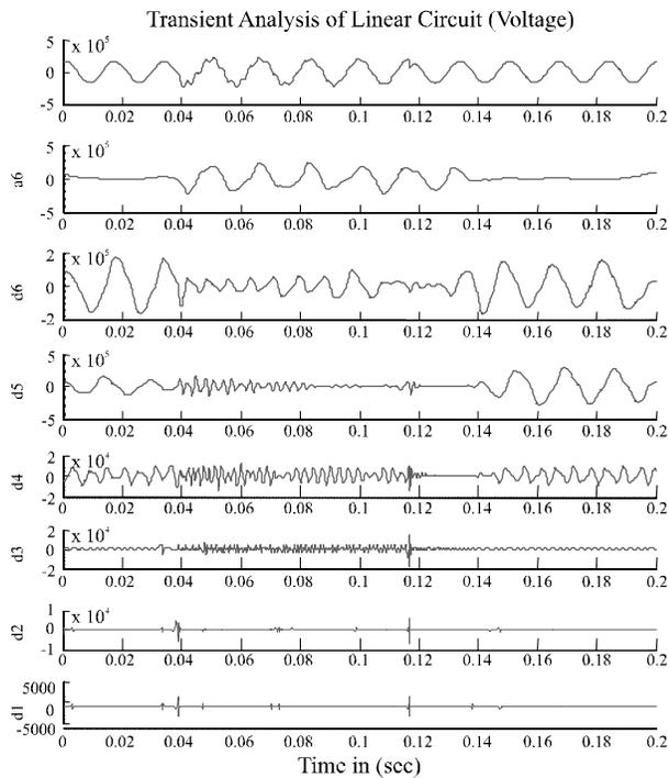
FIG. 5. LINEAR CIRCUIT TRANSIENT SIGNAL WITH  $D_1$ - $D_6$  DETAIL AND APPROXIMATION  $A_6$  COEFFICIENTS
