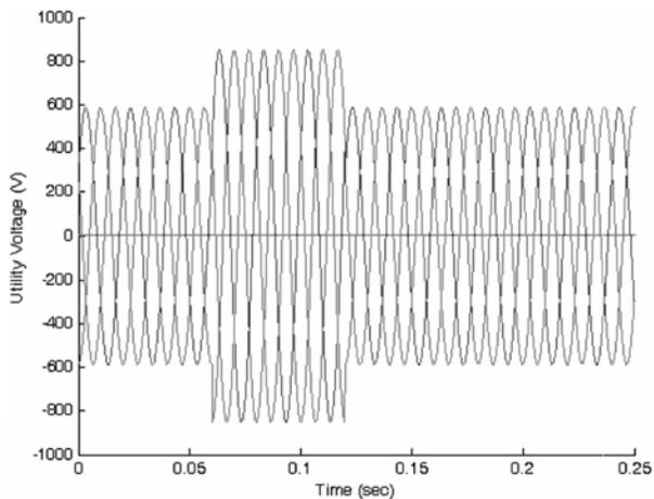
FIG. 15. UTILITY VOLTAGE SHOWING 50% BALANCED 3-PHASE SWELL
