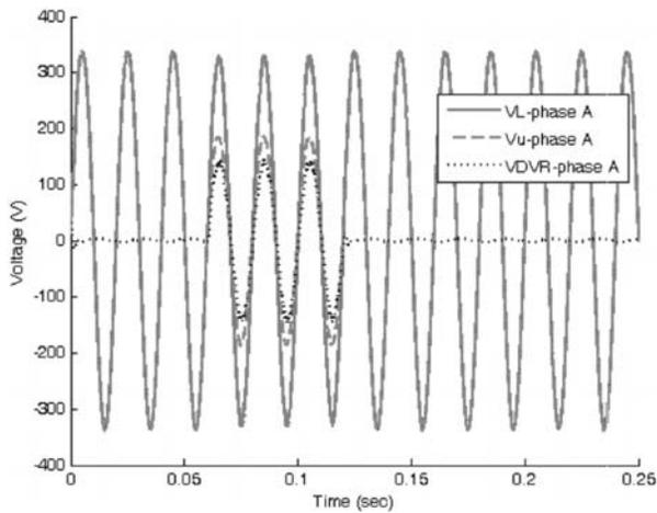
FIG. 12. DYNAMIC VOLTAGES FOR 45% SAG IN PHASE-A OF UTILITY VOLTAGE
