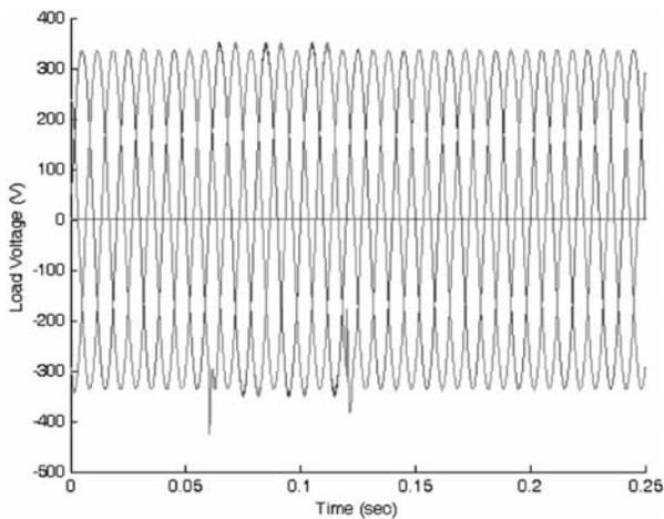
FIG. 18. LOAD VOLTAGE (LINE-TO-GROUND) AFTER COMPENSATING 45% SWELLS ON 2-PHASES
