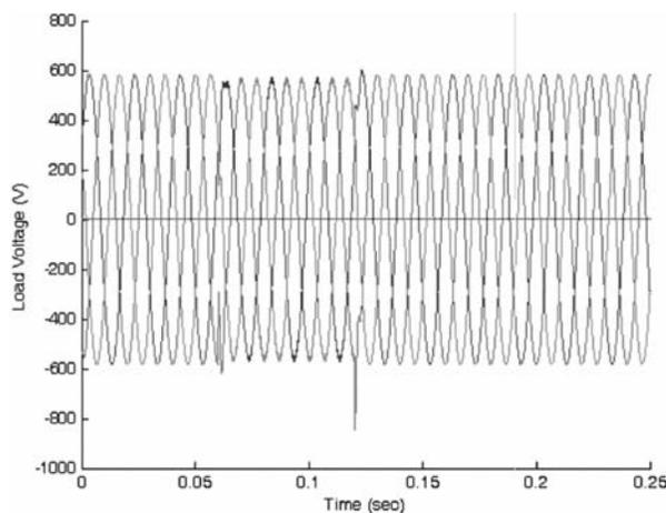
FIG. 8. LOAD VOLTAGE AFTER COMPENSATING A 3-PHASE 50% BALANCE SAG
