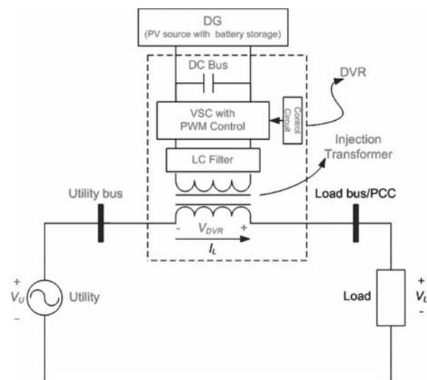
FIG. 1. SCHEMATIC DIAGRAM OF A DVR WITH ITS MAIN COMPONENTS
