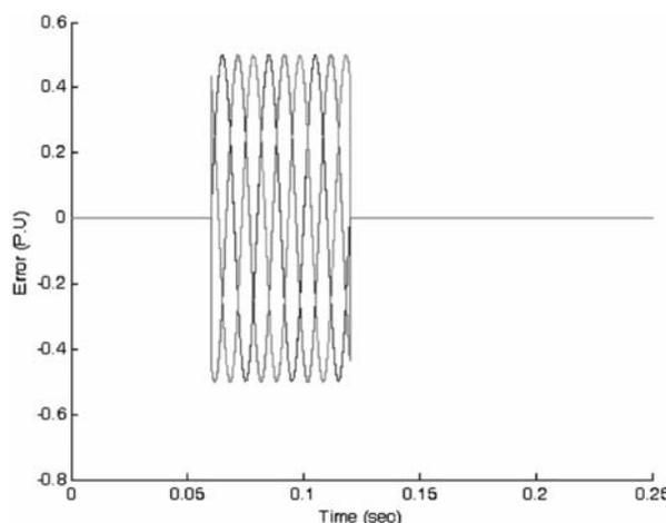
FIG. 7. GENERATED ERROR SIGNAL FOR A 50% BALANCED SAG ON ALL 3-PHASES OF UTILITY VOLTAGE
