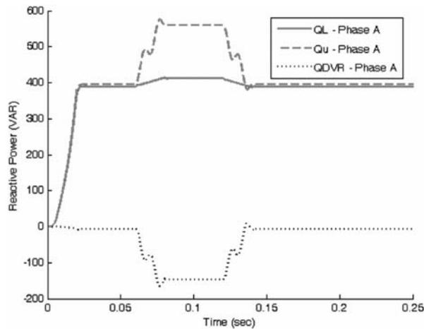
FIG. 21. DYNAMIC REACTIVE POWERS FOR 45% SWELL IN UTILITY VOLTAGE
