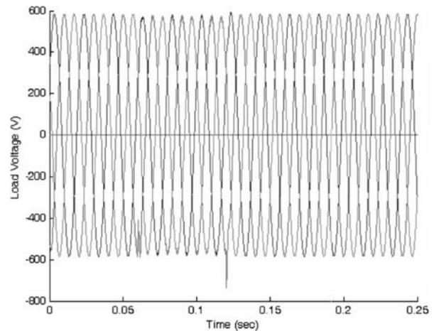
FIG. 9. LOAD VOLTAGES AFTER COMPENSATING AN UNBALANCE SAG ON ALL 3-PHASES
