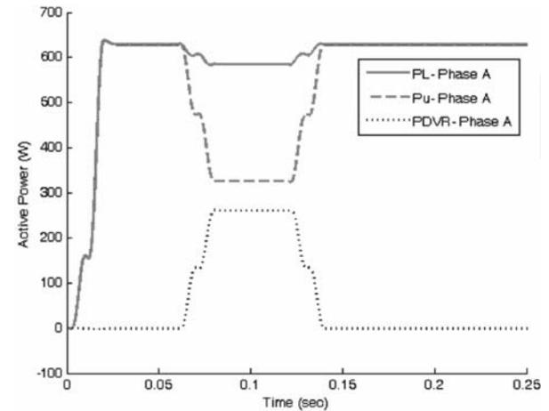
FIG. 13. DYNAMIC ACTIVE POWERS FOR 45% SAG IN PHASE-A OF UTILITY VOLTAGE
