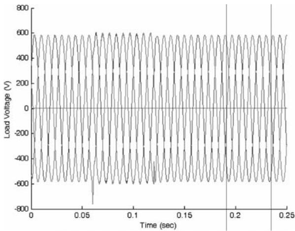
FIG. 17. LOAD VOLTAGE AFTER COMPENSATING AN UNBALANCED SWELL IN 3-PHASE UTILITY VOLTAGE
