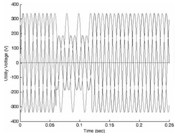
FIG. 10. UTILITY VOLTAGE SHOWING 45% SAG ON 2-PHASES
