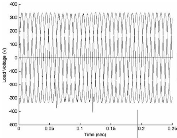
FIG. 11. LOAD VOLTAGES AFTER COMPENSATING 45% SAG ON 2-PHASES OF UTILITY VOLTAGE
