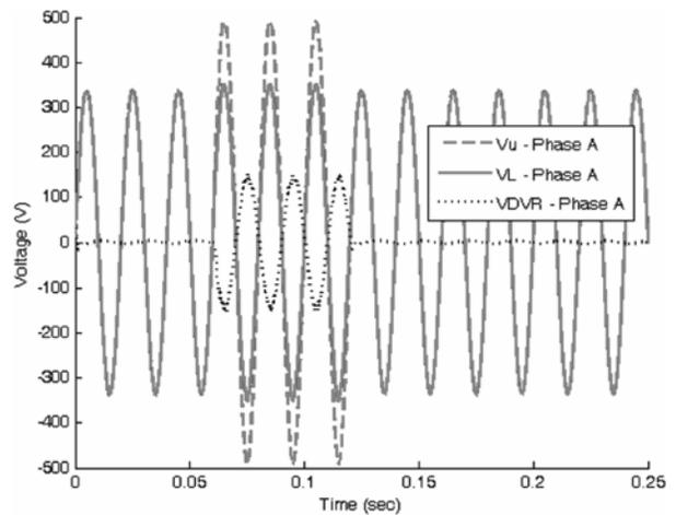
FIG. 19. DYNAMIC VOLTAGES FOR 45% SWELL IN PHASE-A OF UTILITY VOLTAGE
