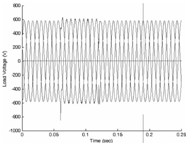
FIG. 16. LOAD VOLTAGE AFTER COMPENSATING A 50% BALANCED SAG ON ALL 3-PHASES OF UTILITY VOLTAGE
