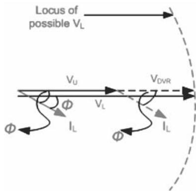
FIG. 2. PHASOR DIAGRAM SHOWING IN-PHASE INJECTION TECHNIQUE FOR A SYSTEM
