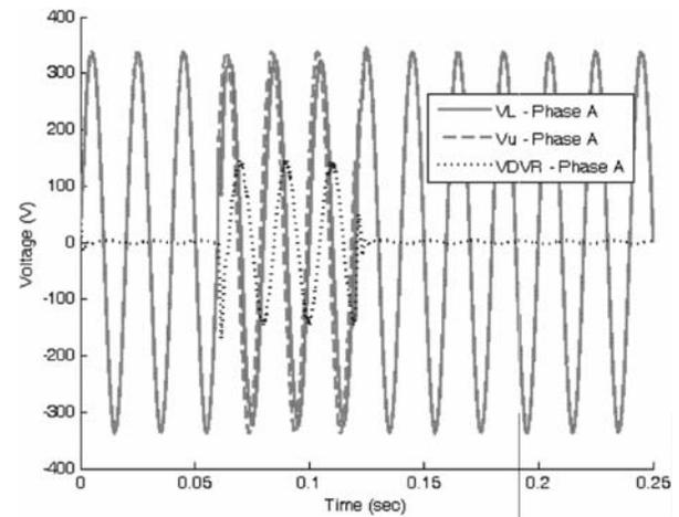
FIG. 22. DYNAMIC VOLTAGES FOR  $+25^\circ$  PHASE JUMP IN PHASE-A OF UTILITY VOLTAGE
