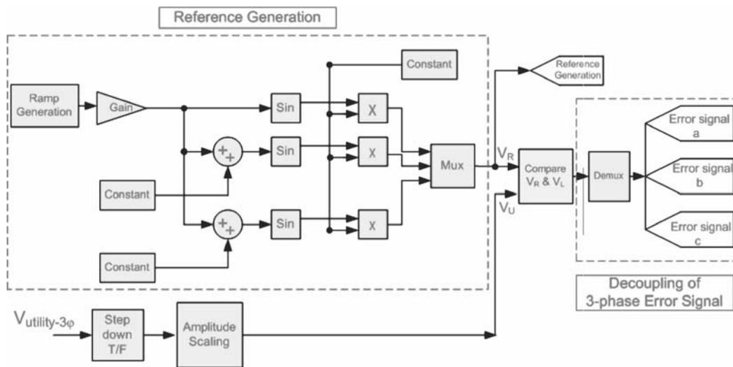
FIG. 4. BLOCK DIAGRAM REPRESENTATION TO GENERATE ERROR SIGNAL
