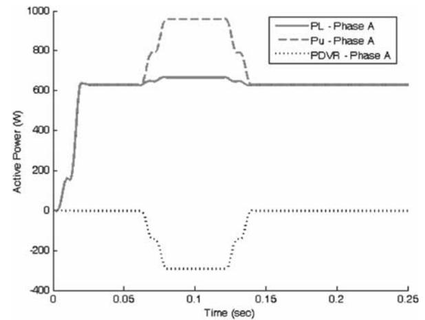
FIG. 20. DYNAMIC ACTIVE POWERS FOR 45% SWELL IN UTILITY VOLTAGE
