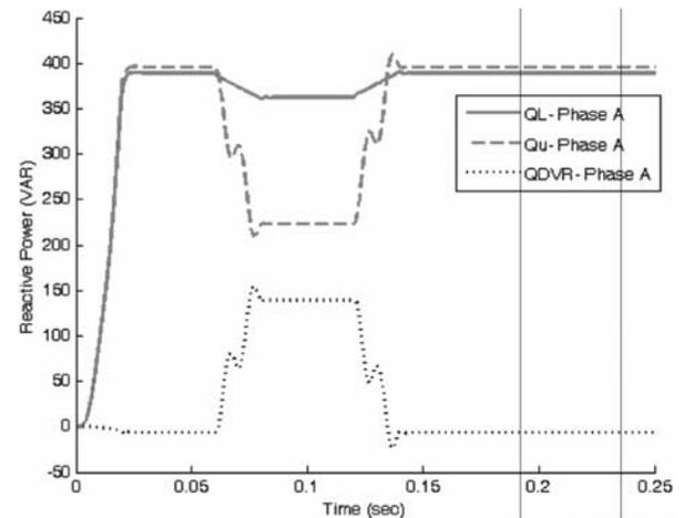
FIG. 14. DYNAMIC REACTIVE POWERS FOR 45% SAG IN PHASE-A OF UTILITY VOLTAGE
