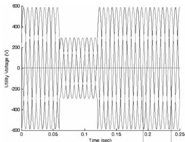
FIG. 6 . THREE-PHASE 50% BALANCED SAG IN UTILITY VOLTAGE
