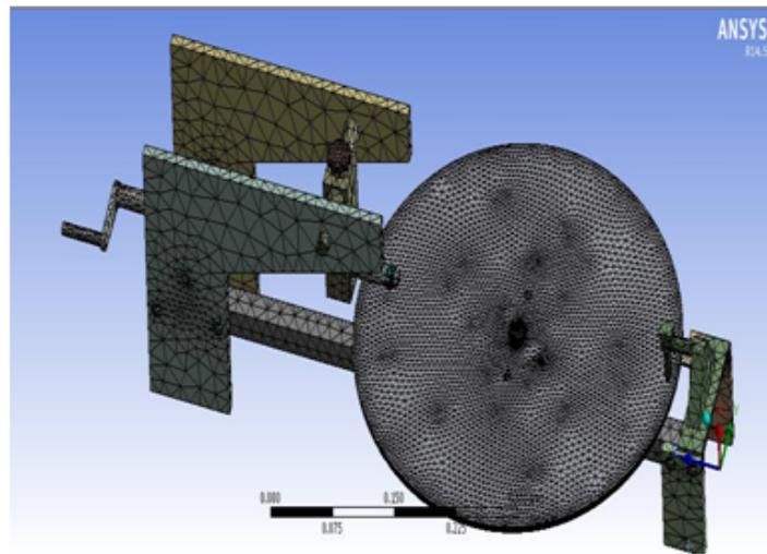
**Fig. 4** – Meshing of the designed part (Ansys workbench).
