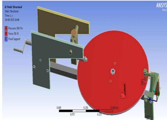
**Fig. 5** – Boundary condition given to the design (Ansys workbench).
