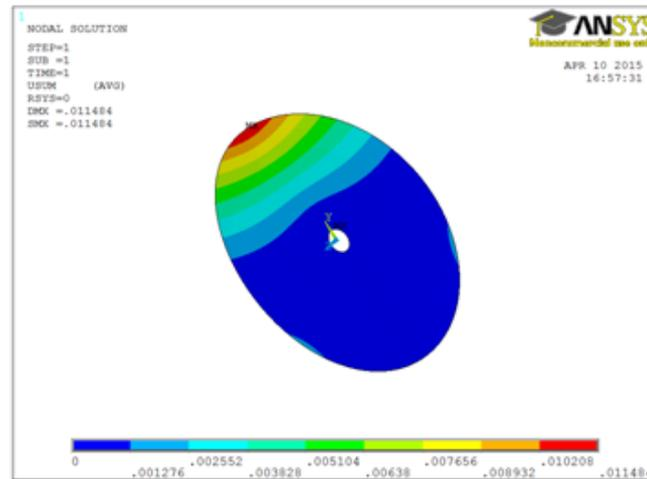
**Fig. 10** – Deformation of the disc (Ansys APDL).
