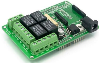
Gambar 4. Modul relai 4 channel ( http://www.emartee.com/ )
