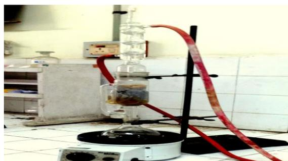
Extraction of pectin by using Soxhlet apparatus
