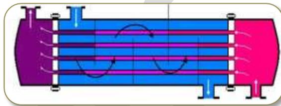
Figure 1: Shell and Tube Type Heat Exchanger
