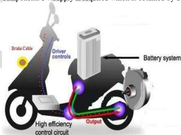
The scooter has a maximum speed of 35km/hr and it is provided with an inbuilt BLDC controller which makes the working of scooter more smooth, silent and efficient.
