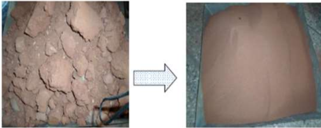
Figure 3 Before and after pulverizing the earth sample
