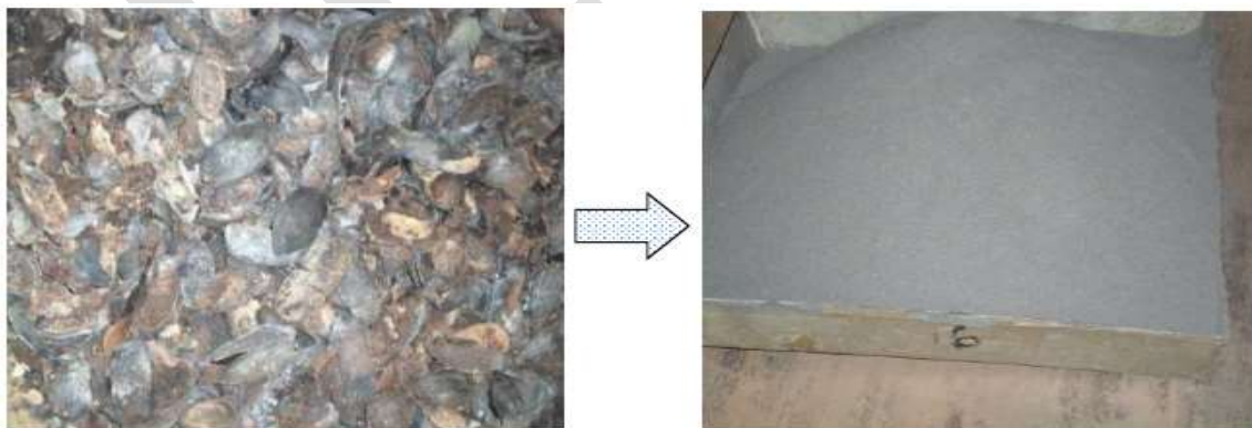
Figure 4 Dried Cocoa Pod Husks before and after combustion
